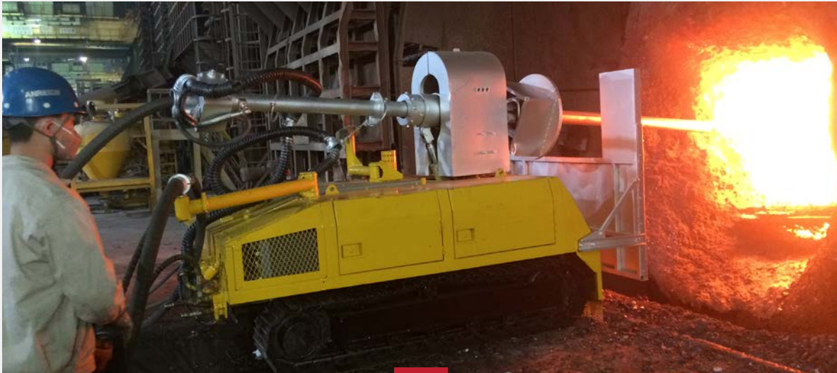
Gunning Robot for HOT REPAIR FOR EAF, Ladle, RH
