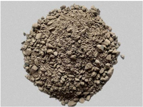
Dry ramming for Bottom
